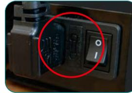
Unplug the power cable from the chair itself. You will find the cartridge containing the main fuse between the power cable and the main switch.
