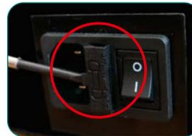
Use a small flathead screwdriver to carefully unhook the fuse cartridge and pull it out.
