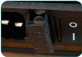
Push the cartridge with the exchanged fuse back into place.
