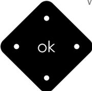
**4-Way-Direction:** This button allows you to navigate within the menu display in four directions. Confirm your selection by pressing "OK".
