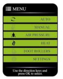
By pressing the **Menu-Button** (12) on your control panel you can now navigate through the different options. You can make individual adjustments to the available functions. Press "OK" after each selection. Press the Menu-Button again to leave the Menu display.
